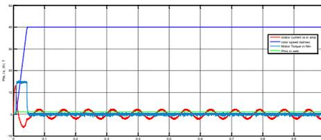
**Fig. 10 Rotor Speed, Motor Torque, Stator Current and Stator Flux magnitude results of SVM-DTC.**
