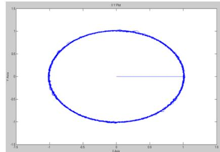
**Fig. 9 Stator flux vector of SVM-DTC**
