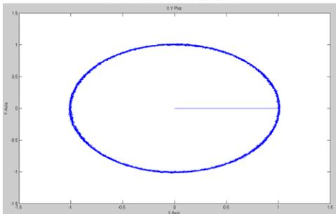
**Fig.13 Stator flux vector of MRAS observer based SVM-DTC**
