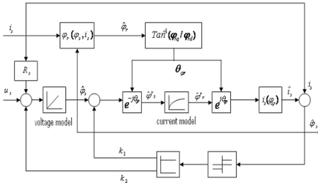
Fig.4 Sliding Mode Flux Observer.
