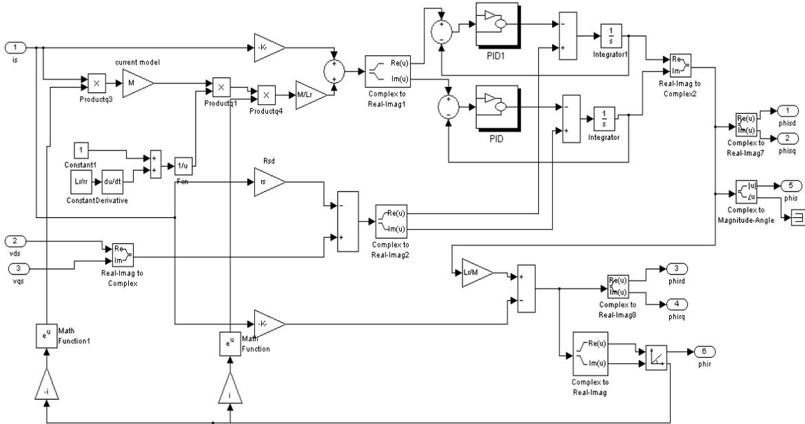
Fig.5 MRAS flux observer simulation diagram
